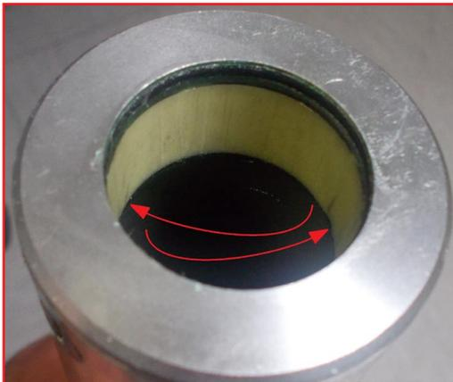
Insert grease under the edge of motor housing
